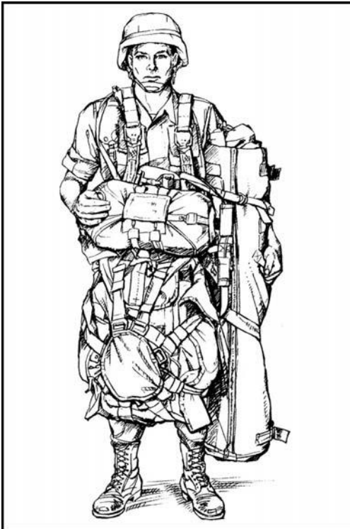
Figure 12-44. DMJP attached to parachutist.
