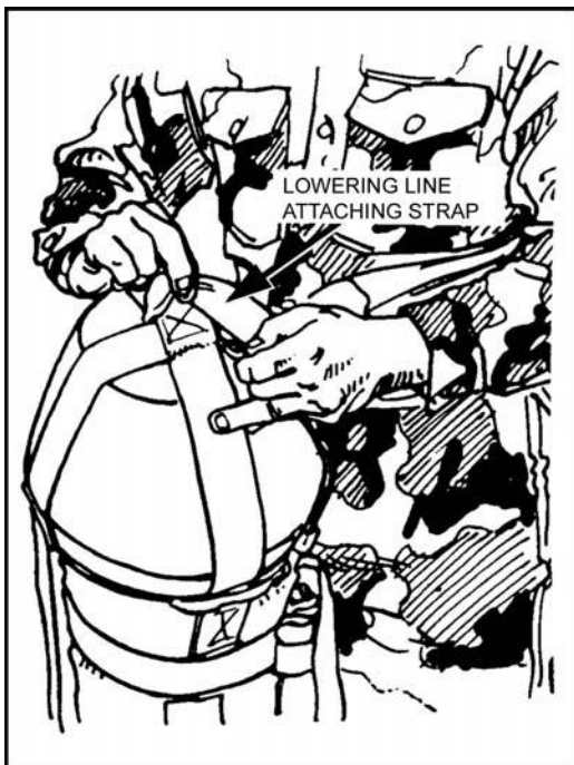
Figure 12-35. Lowering line attaching strap installed.
