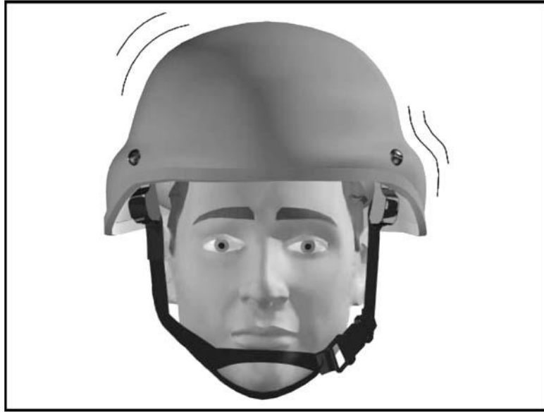
Figure 2-21. ACH too loose.
