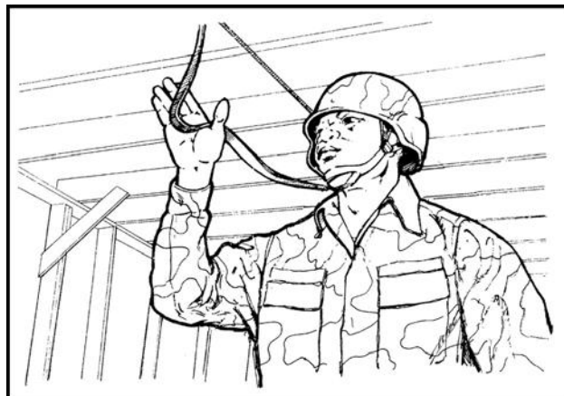
Figure 4-7. Static line bight.
