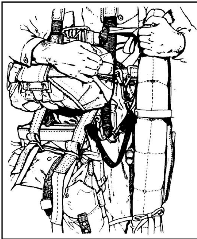
Figure 12-8. Lowering line attached for tandem rigging.
